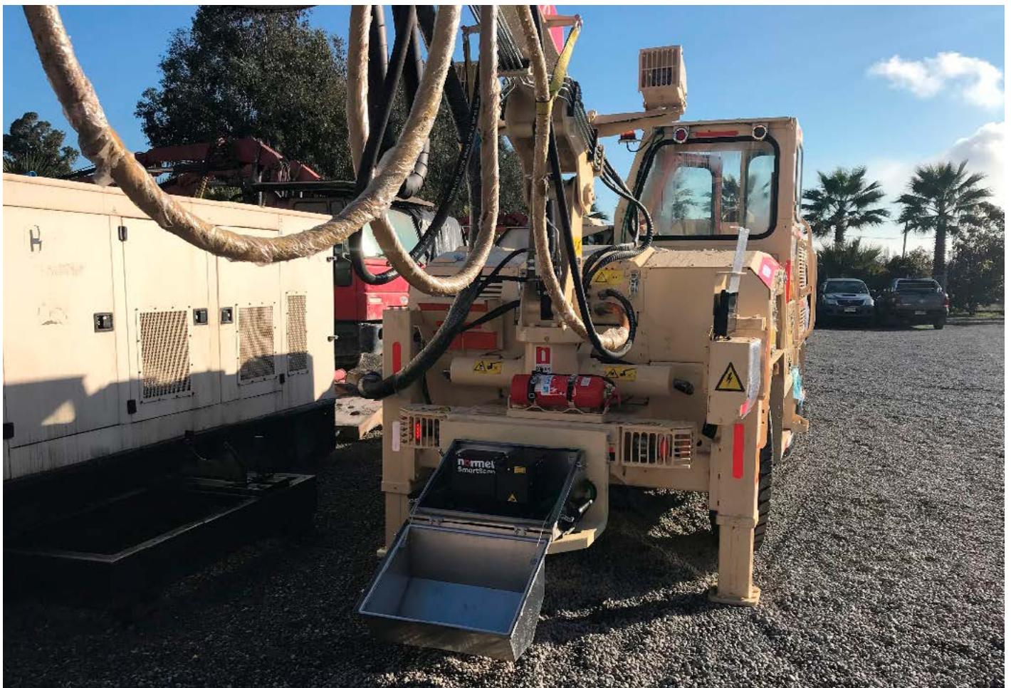
SmartScan retrofit kit installed on Normet Alpha 30.
