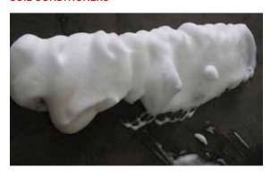
Soil conditioners allow cutterhead torque to be reduced and ensure that the working chamber is filled regardless of the geological conditions present.
